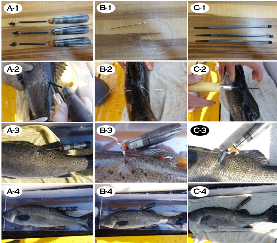
Fig. 1. Three different attachment methods for attaching biologgers to spotted sea bass Lateolabrax maculatus applied in this study: Anchor attachment (AA; A-1 ~ A-4) type, monofilament attachment (MA; B-1 ~ B-4) type and silicone tube attachment (SA; C-1 ~ C-4) type.
